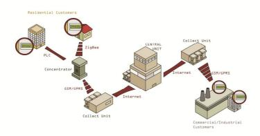
Being developed to meet DLMS, our concentrator can be a part of any AMM system, on the same standard. This characteristic enables our systems to interoperate with all others with similar functions and characteristics, meeting modern requests of DLMS.
